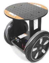
Figure 2 Segway based the RMP (robotic-mobility platform) on the company's personal-transporter product, and it is available in several configurations to support different payload and terrain scenarios.
