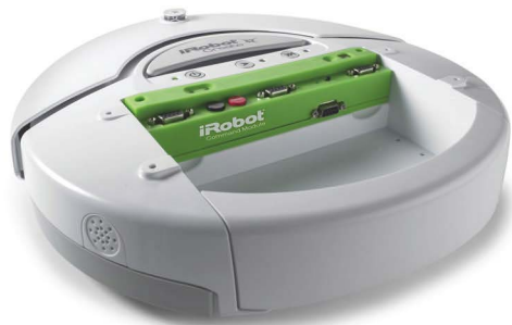
Figure 1 Robot manufacturer iRobot based its Create on the company's Roomba vacuuming robot, and it is available for educators, hobbyists, and developers to add their own hardware and software to control the platform.
